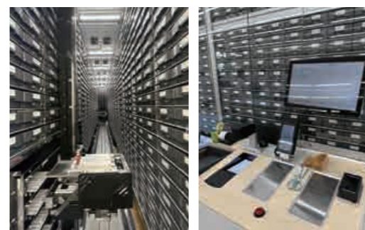
Drug Station, automated medicine picking equipment, introduced to increase customers' safety, improve our productivity, and reduce the waiting time
